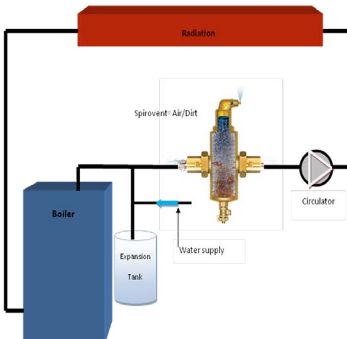
VDR models must be mounted in a straight run of horizontal piping in a perfectly upright position to allow the vent to operate freely. "X" pipe diameters of straight run before and after the unit are not required.
